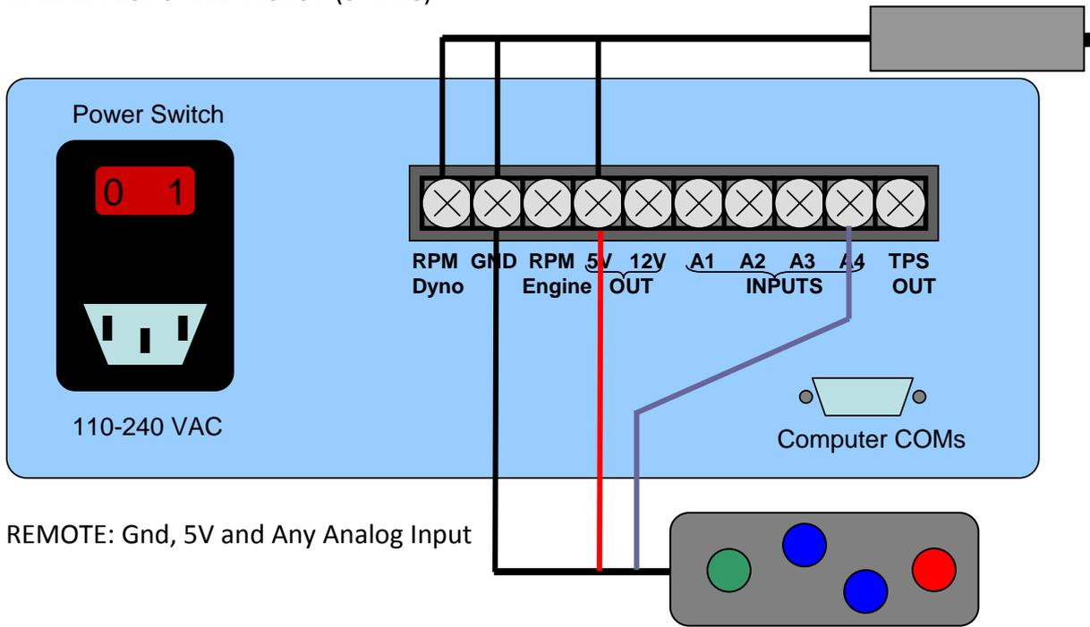
REMOTE: Gnd, 5V and Any Analog Input
