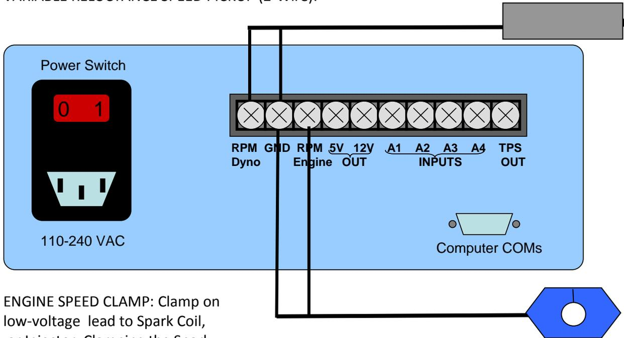
ENGINE SPEED CLAMP: Clamp on low-voltage lead to Spark Coil, or Injector. Clamping the Spark High Voltage line may give "noisy" readings unless Wire is Secured Tightly within clamp. Use Foam or similar to prevent motion of Spark Wire.
