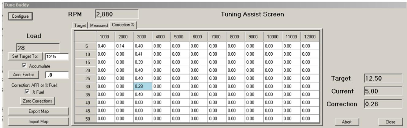
**TARGET:** This is the target AFR. It can be set by entering a number in the upper left box and hitting “Set Target To” button. If you want different target values in different cells, you can Export, edit and then Import the map.
