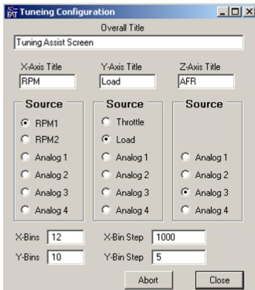
You can select the variable for the X axis, Y axis and Z, as well as the number of bins in the X and Y directions, and their step size. These parameters are saved in the Tune Configuration file.
