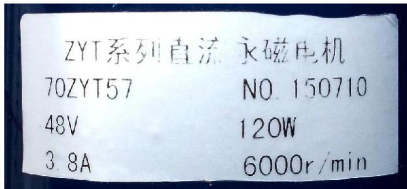
This placard states that it is a 120W (nominal power rating), 48V motor designed to operate at 6000 rpm. The current draw is listed as 3.8A at 48V. Electrical power is current times voltage:
