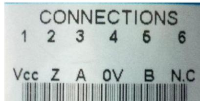
Pressure sensors connector (viewed facing to connector on DAQ)
