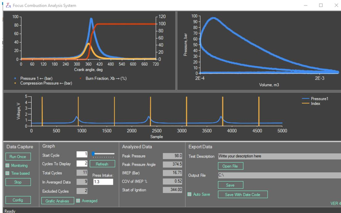
Different analysis parameters can be added to the upper right graf by clicking the Grafic Analysis button at the bottom of the screen. These calculated curves depend on the measured pressure trace, and the various input parameters, such as Engine Geometry, Intake pressure and Temperature and polytrophic Coefficient.
