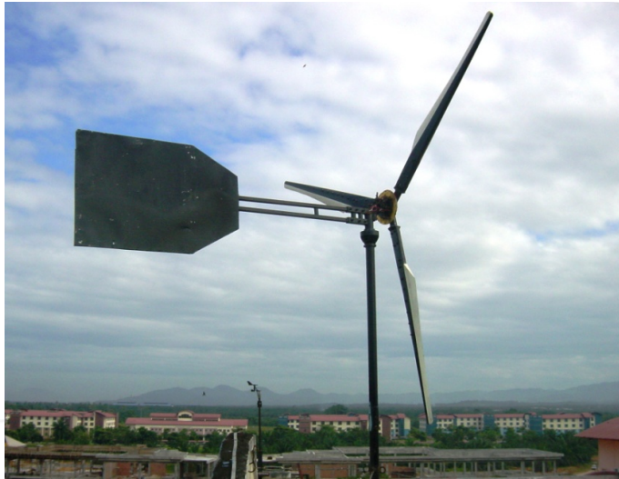
Figure 10. Wind turbine with optimized generator during turbine evaluation. Notice the anemometer in the background to the left.
