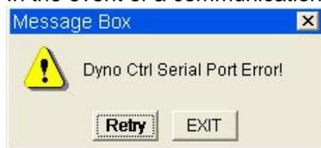
If this appears it means that the software was unable to communicate with the dynamometer controller through the designated port. This is generally the result of one of the following:
