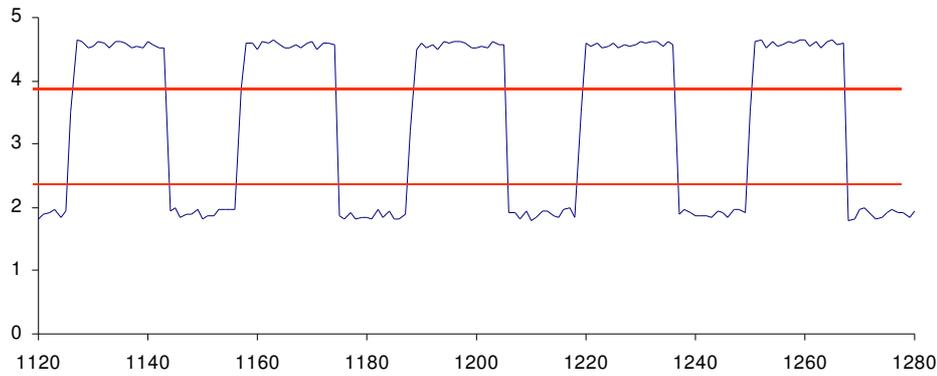
For AC type sensors, such as Variable Reluctance (magnetically inductive) sensors, the signal drops below 0V, and may go up to several tens of volts. The triggering circuitry is designed to accept this wide range of signal voltages without harm. For AC sensors it is common to set the Lower Trigger Level at 0.5V, and the upper Trigger Level at 1.0V. It is easy to determine the appropriate voltage levels by viewing the signal on an oscilloscope.
