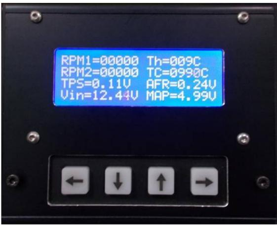
In normal operation several parameters are displayed on the screen with or without the SD card present. These include RPM1 and RPM2, TPS, Vin (ie. the 12V power source), Thermistor temp (Th), Thermocouple temp (TC), AFR and MAP.
