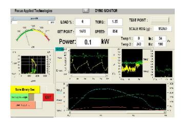
This 5th generation dynamometer controller is a universal dynamometer controller for all eddy current and generator type dynamometers. With optional Hydraulic Servomotor it can run hydraulic and Water Break dynamometers as well. A Throttle Position sending control is provided from the front panel, and with optional throttle control servomotor can control the engines throttle.
