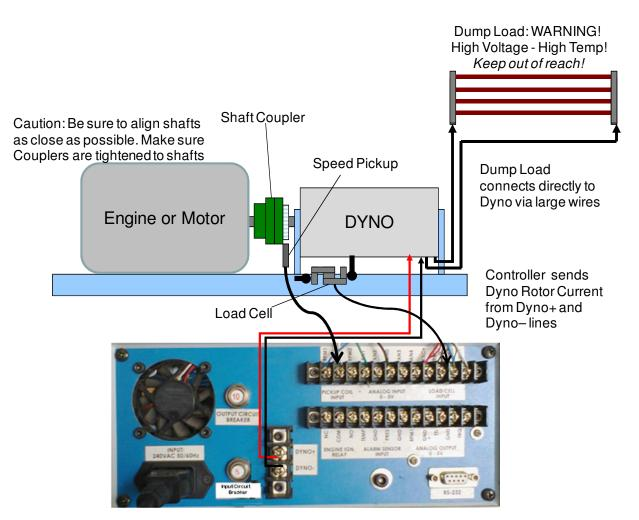
The Controller unit is powered from a clean AC line power source.
