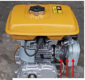
Supply air flow to cold down carburetor, especially during prolong low speed high load test
