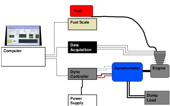
The Dynamometer and Dynamometer Controller together with the engine form a complete system. The Dyno controller reads the speed and torque from the dynamometer and controls the load according to its mode and set point. Power extracted from the engine is dissipated as heat in the dump load.
